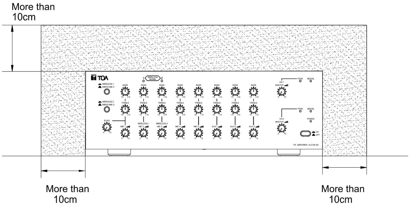
This amplifier is designed for portable use and not for rack-system mounting.
