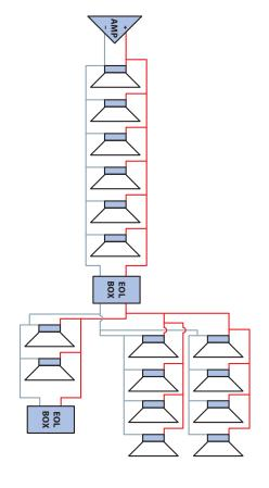
**Note:** that some loudspeaker circuits are extremely reactive and very electrically complex. Some impedance measurement and analysis may be required to achieve a predictable measurement.
