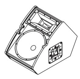
panel with dual NL4 connectors is located on the rear of the enclosure, which keeps the connectors hidden and away from the performers on stage.
