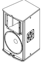
The TX1152 from Electro-Voice is a high power, high sensitivity, 2-way loudspeaker system that can be used in a variety of applications where high quality sound reinforcement is required in a lightweight package. The TX1152 utilizes the DH3, a high output 1.25 inch titanium compression driver, coupled to a Constant Directivity 60° x 40° horn. This combination results in a smooth response to 20 kHz and excellent pattern control in medium throw applications.
