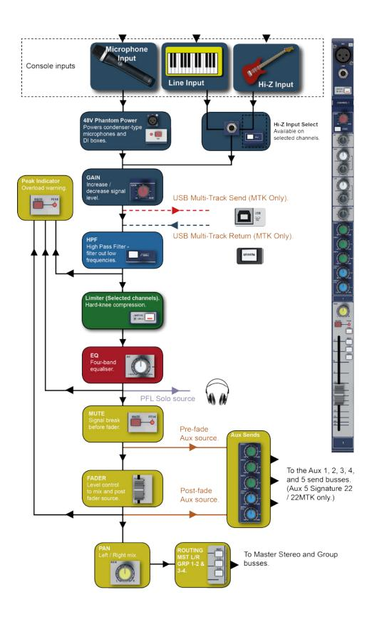
All mono input channels have the choice of XLR (mic) and Jack (Line) balanced inputs; the two highest numbered mono channels have Hi-Z input switches for the line inputs while channels 1 and 2 incorporate switchable input limiters.
