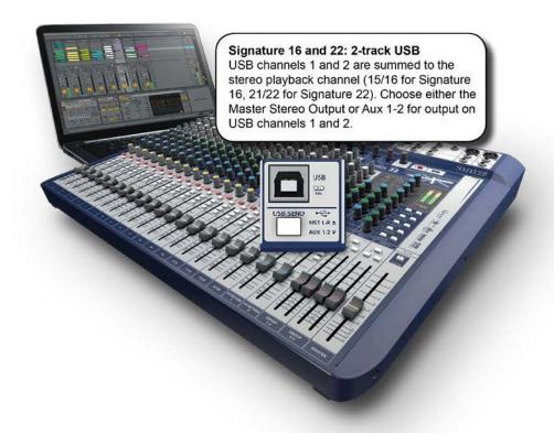
The Signature 16 and 22 consoles have 2-track USB input and output functionality. This could be used for recording a mix to a PC or Tablet, for example - or to use a computer as a playback device. Channels 1 and 2 are received by the Stereo Playback Channel (15/16 for Signature 16, 21/22 for Signature 22).
