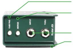
**-15dB PAD** reduces input sensitivity for active high-output instruments.
