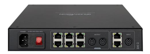
The Soundvision DCS-1000EX is used to extend the power supply of the speaking unit, and it acts as a relay when the power supply of the controller is insufficient. Support 1 group of 2-way RJ45 interface and 1-way 8-pin interface input, 2 groups of 4-way RJ45 interface and 2-way unit output of 8-pin interface, can be connected to the speaking unit.
