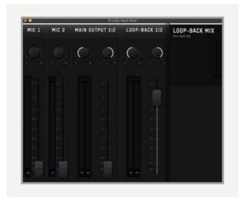
This enables you to blend from both the Mic and DI Inputs as well as the playback of your computer all into a summed signal stereo feed by pulling up faders of the various channels to create a mix. This stereo feed/mix can then be recorded or streamed. The channels are as follows:
