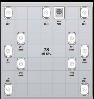
Systems can be level calibrated in compliance with the latest broadcast and film standards. and delay is inserted per monitor to compensate for differences in distance to the listening position. Finally, one or more subwoofers can be added, and the entire audio system guickly adjusted for personal spectral preferences if
