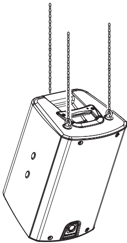
Suspension using M10 shoulder eyebolts.
