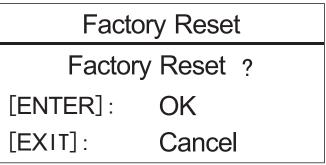
2. Press the [ENTER] button (press [EXIT] return to the previous interface), to return to the default factory settings.
