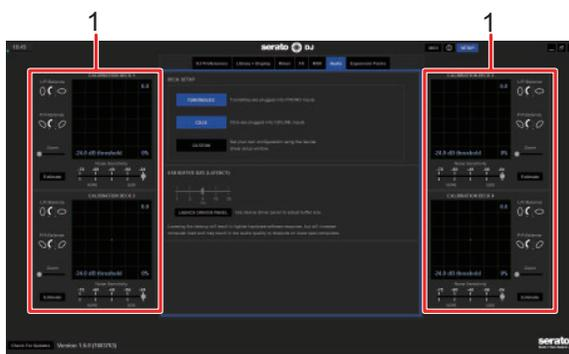
1. **CALIBRATION DECK:** Serato DJ Pro calculates analog signals from a control disc and processes the signals for digital audio files. It calculates signal levels and device statuses for each operating environment and sets up optimal settings for reading the control signals.
