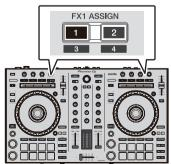
Press the [FX ASSIGN] 1 button to assign the effect to deck 1, the [FX ASSIGN] 2 button to assign the effect to deck 2.
