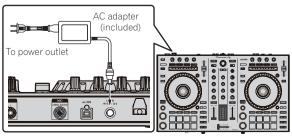
6 Press the [STANDBY/ON] switch on the rear panel of this unit to turn this unit on.
