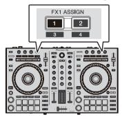
Press the [**FX ASSIGN**] 1 button to assign the effect to deck 1, the [**FX ASSIGN**] 2 button to assign the effect to deck 2.
