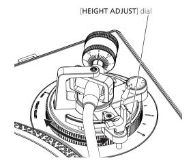
3 Turn the [HEIGHT ADJUST] lock to fix the height of the arm
