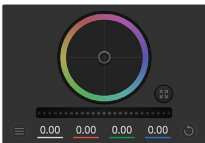
Adjust the master wheels by dragging the wheel control left or right
