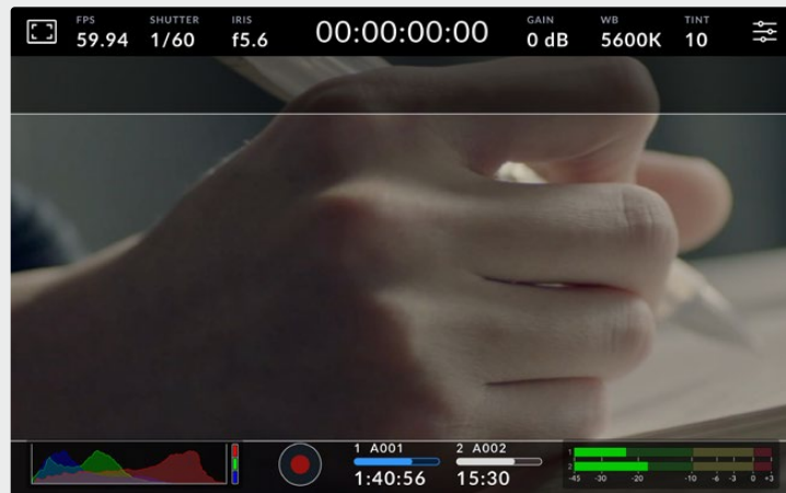
The LCD touchscreen with 2.40:1 frame guides enabled
