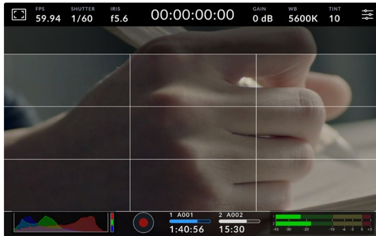
The rule of thirds grid automatically scales to any on screen frame guides
