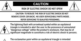
The exclamation point within an equilateral triangle is intended to alert the user of the prescence of important operating and maintaining (servicing) instructions in the literature accompanying the appliance.
