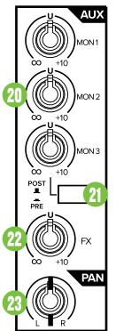
The FX signal reaching the internal FX processor and the FX send output jack is the sum (mix) of all the channels whose aux FX control is set to more than minimum.
