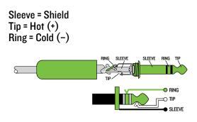
To connect unbalanced lines to these outputs, use a 1/4" mono (TS) phone plug, wired as follows:
