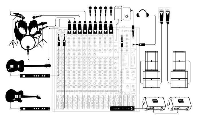
This diagram shows a bass and guitar attached to the channel 1 and 2 line-level inputs, each via a mono effects processor. The Hi-Z switch is engaged on both channels. A mic'd up drum kit utilizes the next four channels of the mixer. Microphones are connected to the following five channels and will handle lead and background vocal duties. A phone is connected to the last channel on the board, the 1/8" stereo input.
