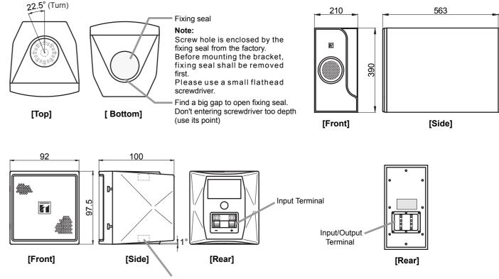
2-M5 Screw holes (top and bottom) (Screw length max. 12mm or 0.47inch)
