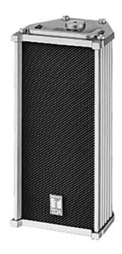
The TZ-105 Column Speaker employs multiple cone speakers arranged vertically on a single baffle board to provide wider horizontal directivity.
