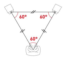
The A8H comes in two versions: left and right. Usually, they are positioned according to the naming (left picture below), however if space is limited, for example in a very narrow room, it is OK to swap the loudspeakers (right picture below). When doing this ensure that the acoustic axis is still positioned with a 60° spacing so that the stereo imaging is unaffected.
