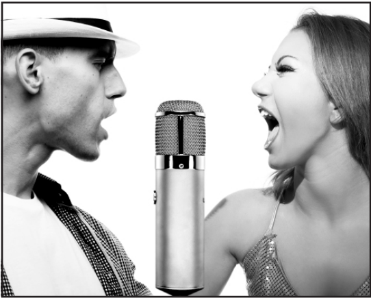
In this image, two vocalist perform at the same time on either side of the WA-47 using a figure-of-eight pattern.
