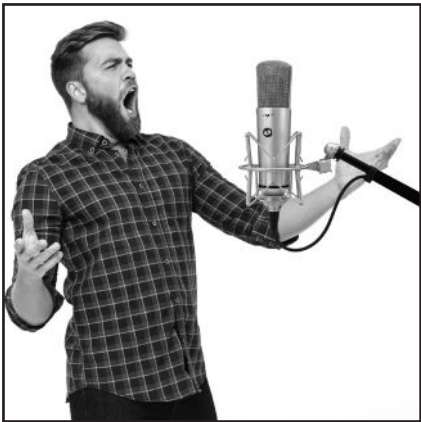
In this image, a vocalist performs into the WA-87 R2 at a distance of 12", in cardioid pattern.
