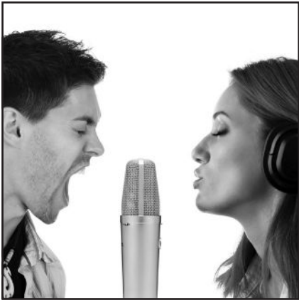
In this image, two vocalists perform at the same time on either side of the WA-87 R2 using a figure-of-eight pattern.
