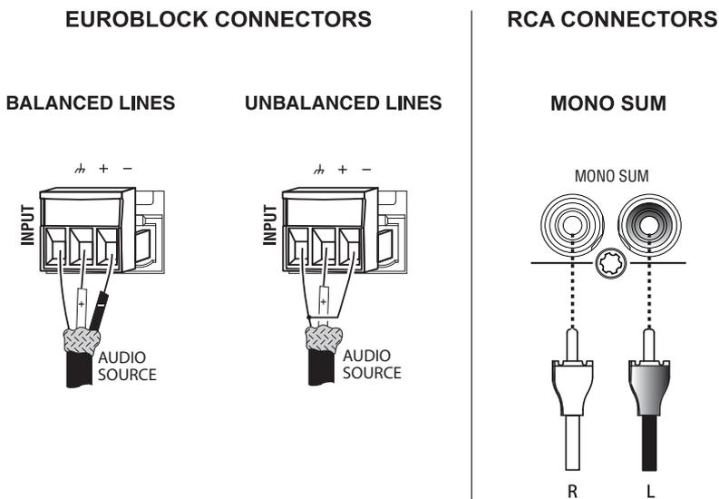
**Note:** Two RCA connectors are provided for summing left and right channels from a stereo source. Do not use both Euro-block and RCA connectors concurrently for any single input channel.
