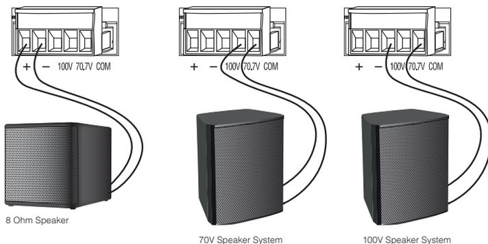
Figure 2.6 Wiring Audio System
