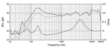
On-axis in half-space (2pi, solid line) and full-space (4pi, dotted line) at thru  $(8\Omega)$  setting Input Impedance
